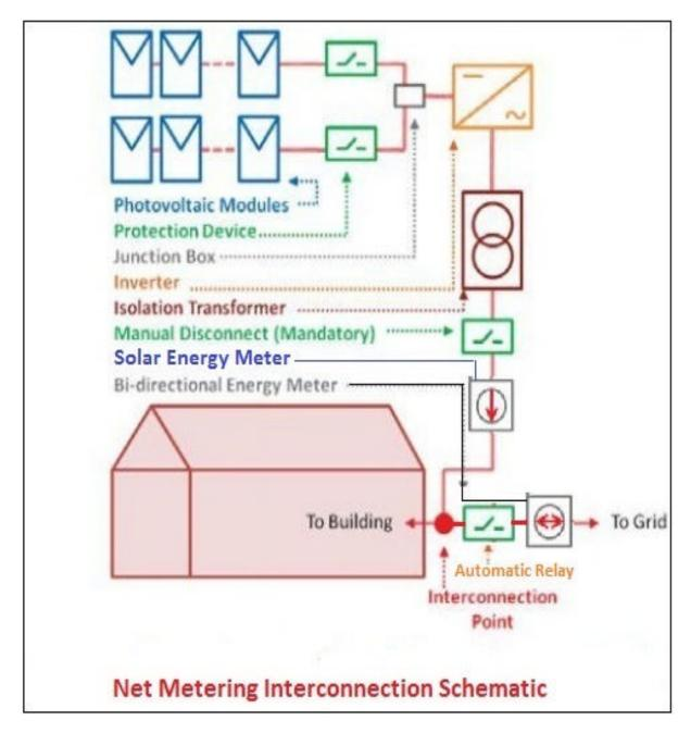
Note: 1) The schematic diagram shown is a model Solar net metering system.
