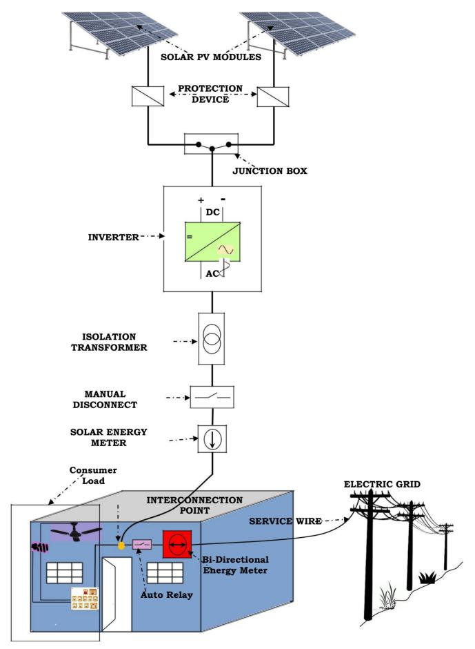
Solar Rooftop PV system HT Net metering Schematic Diagram
