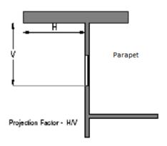
"Projection factor, side fin": the ratio of the horizontal depth of the external shading projection divided by the distance from the window jamb to the farthest point of the external shading projection, in consistent units;
