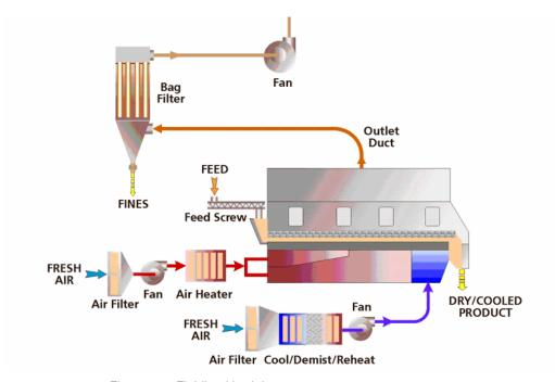
Figure 3-5: Fluidised bed dryer
