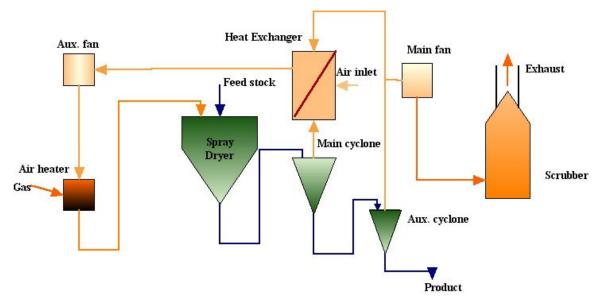
Figure 6-1: Heat recovery- Spray Dryer
