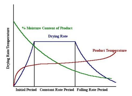
Figure 2-1: Drying Curve
