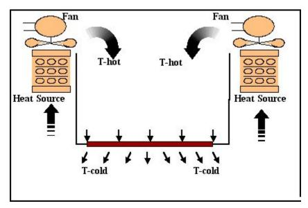
Figure 5-1: Delta T control system for hot air drying
