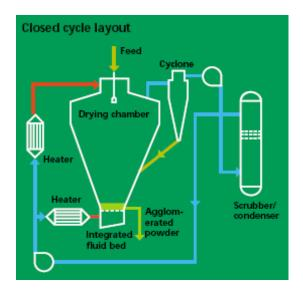
Figure 3-4: Closed cycle spray dryer lay out
