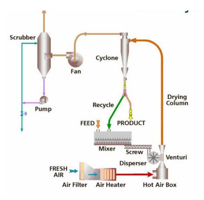
Figure 3-2:Pneumatic /Flash Dryer
