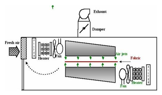
Figure 3-6:Schematic of a stenter
