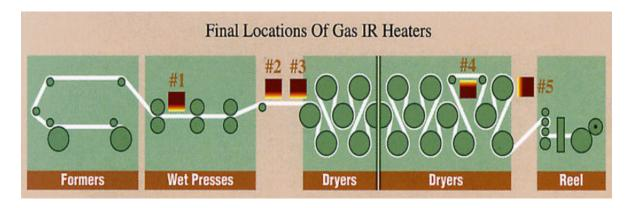
Figure 3-8: Infrared heating for paper machine
