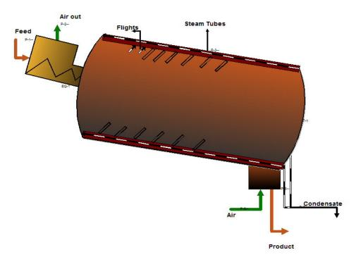
Figure 3-1 Indirect Rotary Dryer
