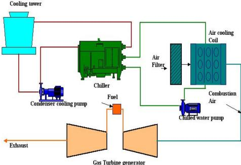
Gas Turbine generator Figure 7-8: Gas turbine inlet air cooling
