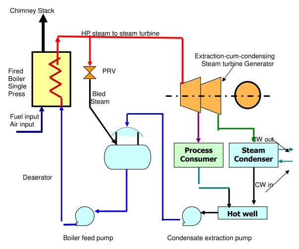
Figure 3-2 Extraction-cum-condensing steam turbine based cogeneration system
