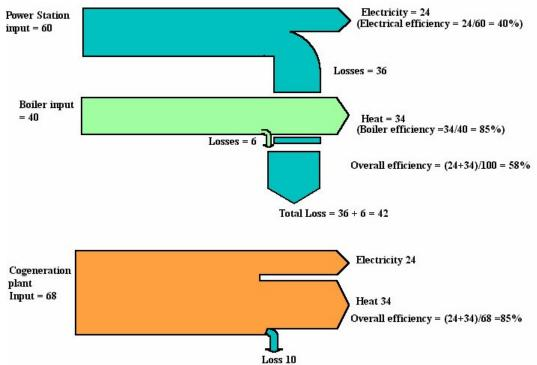
Figure 2-1: Cogeneration (Bottom) compared with conventional generation (top)
