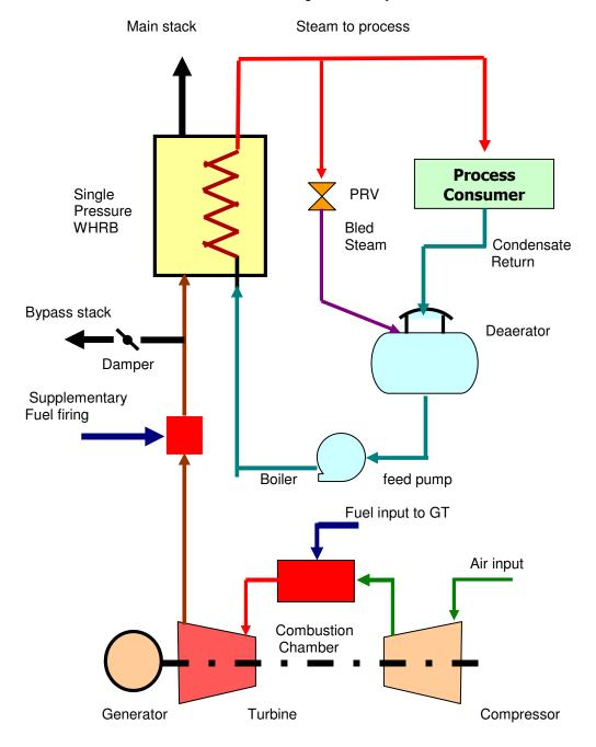
Figure 3-3: Gas turbine based cogeneration system with supplementary fired WHRB
