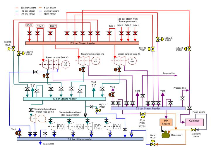
Figure 7-3: Steam Generation & Distribution System
