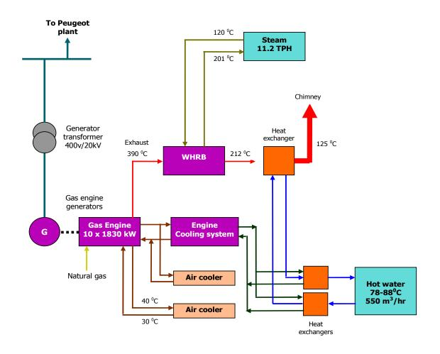
Figure 7-7: Gas engine based cogeneration plant
