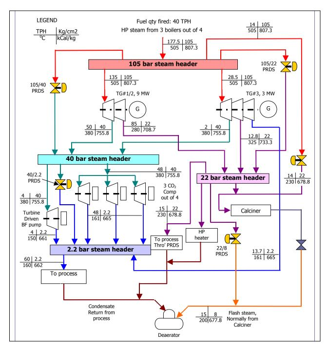
Figure 7-2: Heat balance of Cogen System- Soda Ash Plant
