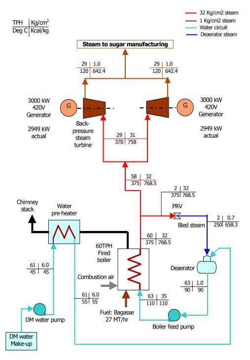
Figure 7-1: Cogeneration system-Sugar Mill
