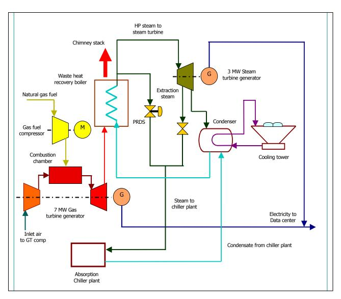
Figure 7-5: Trigeneration-Power, heating and cooling
