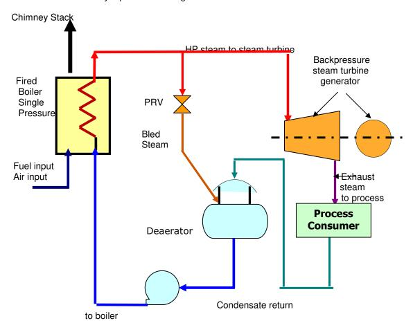
*Figure 3-1: Backpressure steam turbine based cogeneration system*
