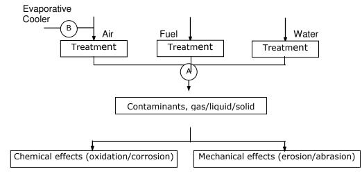
Note: A in circle – Control of total contaminants B in circle – Secondary control of evaporator cooling water
